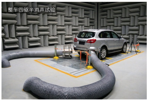
整车四驱半消音室 NVH semi-anechoic lab
